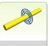
When an electric current runs through a wire, an electromagnetic field is generated around it.
