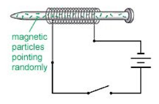
The magnetic particles in a soft iron nail will line up with the magnetic field when the current is switched on.
