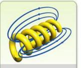
By winding the wire into a tighter coil, the field is made stronger, i.e., higher current and more number of wire turns produce a stronger field.
