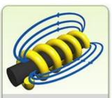
The field can be made stronger by placing an iron bar in the coil center, thus, increasing the power of the electromagnet.
