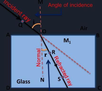
Angle of refraction Refraction of light
