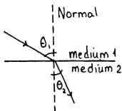
The amount of bending is represented with the letter *n*, which stands for the **index of refraction**. The index of refraction for a particular medium is a ratio of the speed of light in a vacuum to the speed of light in the medium.
