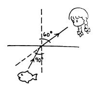
**Solution: a.** The fish will appear to be straight ahead according to Amy. However, because light travels slower in water than in air, the fish is closer to Amy than she thinks.
