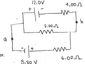
a. Calculate the current in each resistor.
