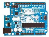
Arduino Uno - The microcontroller development board that will be at the heart of your projects. It's a simple computer, but one that has no way for you to interact with it yet. You will be building the circuits and interfaces for interaction, and telling the microcontroller how to interface with other components.
